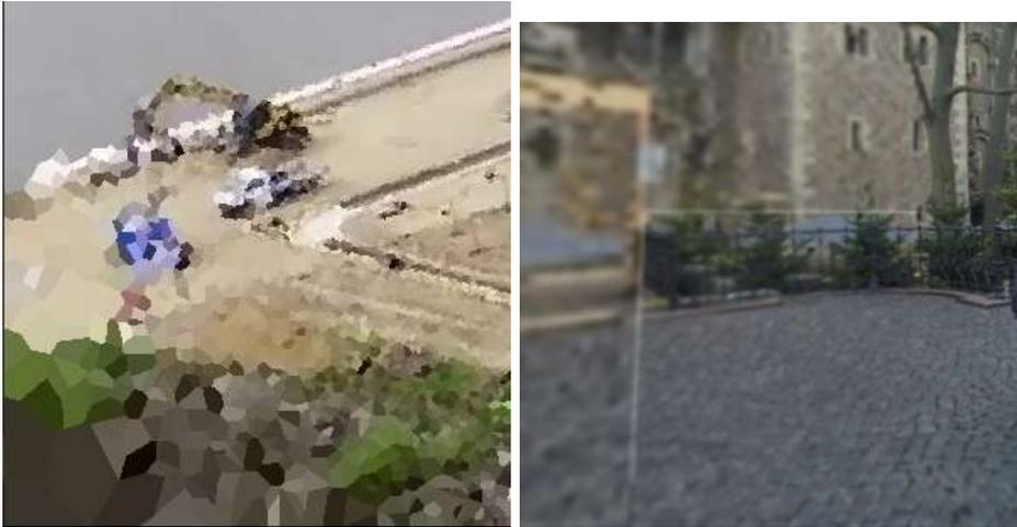
Figure 5.9: Rendering artifacts: These pictures show possible rendering artifacts for both frameworks. Framework 1 (left) has flickering edges due to the interpolation mask. Framework 2 (right) can introduce hard edges relating to the transition between video tiles of different resolutions.
