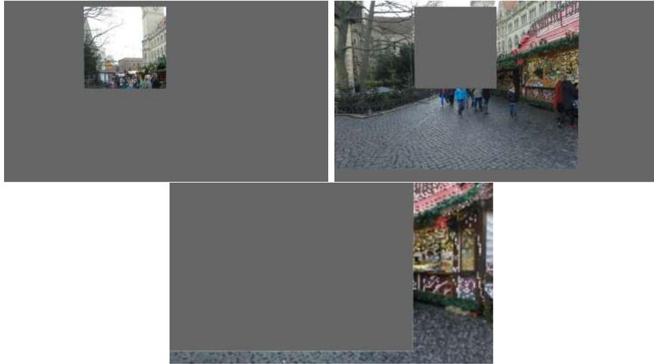
Figure 4.5: Streamed texture levels: For every frame, only updated texture data for every mip-map level are streamed to the GPU. The pictures displaying the transferred cube-map data for the maximum (top left), medium (top right) and lowest (bottom) resolution. The grey area is not updated, and thus either containing data of old frames or being uninitialized.
